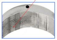
Vane pump cam ring
